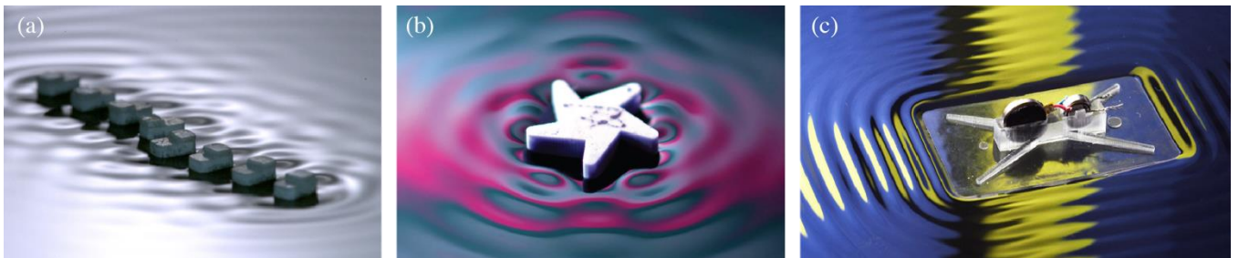
Figure 1 (a) Eight capillary surfers on a vibrating bath organize in an orbital structure, stabilized by their mutual capillary wavefield [1,4]. In isolation, each individual surfer propels at a constant speed along a straight trajectory. (b) A chiral “spinner” steadily rotates on a vibrating bath, propelled by its self-generated capillary wavefield [2]. (c) A “SurferBot” self-propels along a fluid interface, driven by an onboard vibration motor and battery [3].
