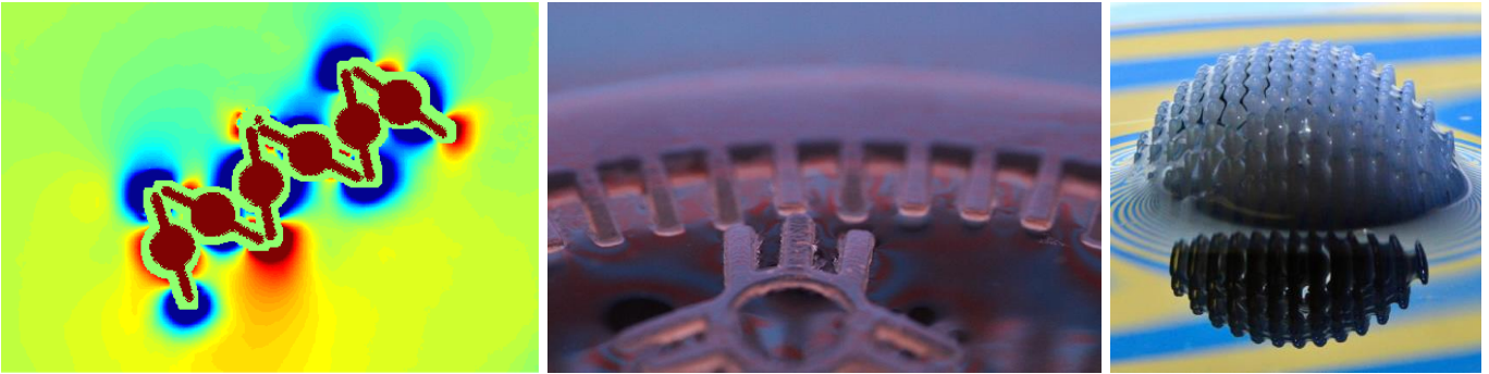
Figure 1 From left to right, illustrations of the self-assembly of floating components. (left) A chain of 6 components possessing positive and negative menisci is self-folding into an undulated floating structure. (center) Positive and negative menisci controlled by the curvature of floating objects allow for complex interactions close to molecular recognition. (right) An array of spines is piercing the liquid interface creating a giant meniscus. If the shape of each spine is judiciously chosen, the shape of the meniscus can be controlled like here in a hemispherical shape.
